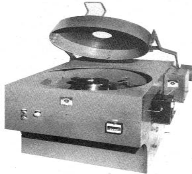
Fig. 2-3. Small vertical-axis casting machine, floor model.
